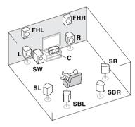
A 7.1 ch surround system connects the left and right front speakers (L/R), the center speaker (C), the left and right front height speakers (FHL/FHR), the left and right surround speakers (SL/SR), the left and right surround back speakers (SBL/SBR), and the subwoofer (SW).
